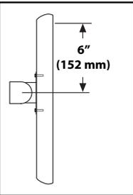
EN Mounting height assumes there is a 6" (152 mm) distance between the center of your monitor mounting holes and the top of the screen. If your distance is smaller, you should increase mounting height accordingly, if your distance is larger, you should decrease your mounting height accordingly.
