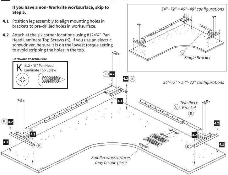
**4.3** With frame set positioned and the six corner screws secure, attach the frame set using the remaining #12×3/4" Pan Head Laminate Top Screws (K).
